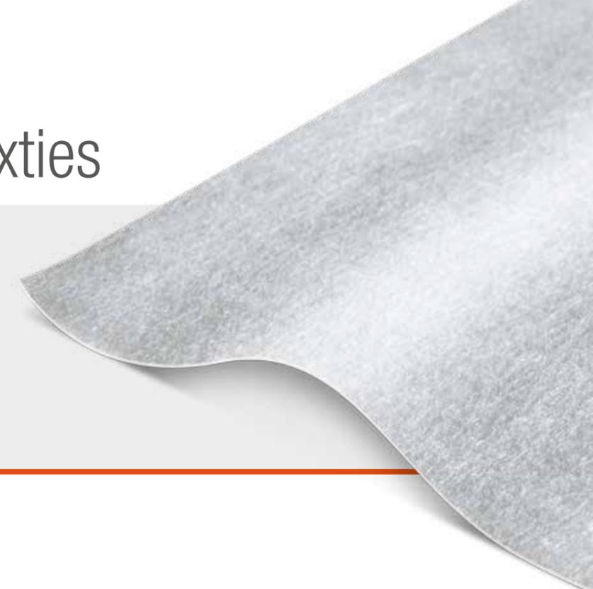
**TERRAM Standard Geotextiles enhance the performance and design life of granular layers by providing the filtration and separation functions. Typical uses for TERRAM Standard Geotextiles include ground stabilisation (between the sub-base and subgrade) and around drainage materials.**
