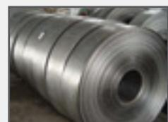
D. Electro Galvanized Steel (Electrolytic Coating) DC01 + ZE,
